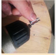
Set your drill depth. Make sure it won't drill right through the table surface. Pre-drilling holes in your marked spots will save you from splitting the wood.
